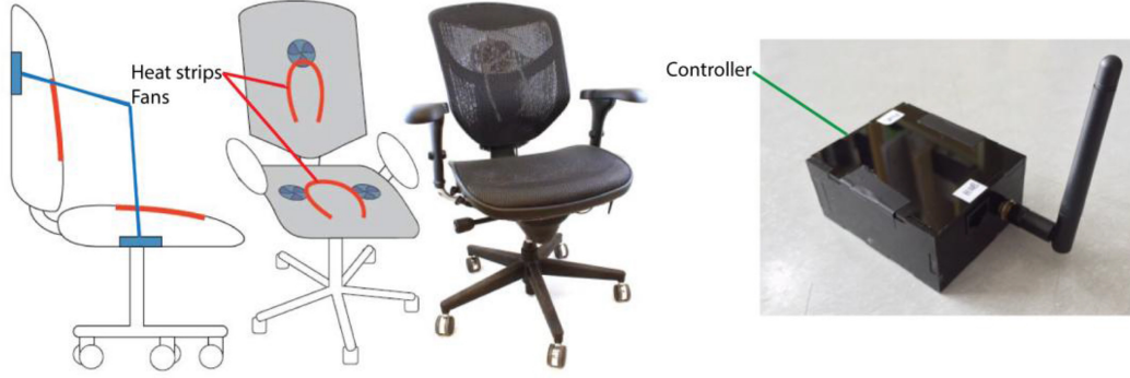
Figure 2.1: This image from [83] shows heating and cooling elements of the personal comfort system (left side) and the controller with wireless connectivity (right side).
